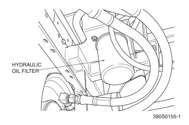
Figure 7-3. Hydraulic Oil Filter
